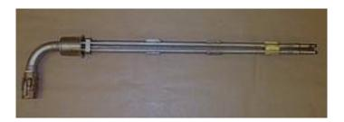
Both the metallic and the refractory parts of the burner are cooled by the oxygen flow. Experimental and modeling studies have been carried out to design the inner shape of the burner in order to ensure efficient cooling and to prevent any deposit forming inside the block.
